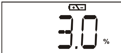
Figure 3: Low Battery Condition
